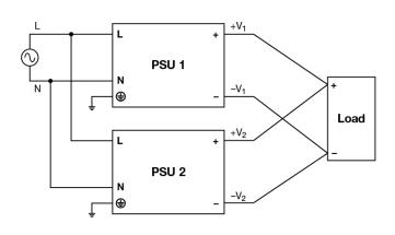
Fig. 6 Parallel Operation Connection Diagram
