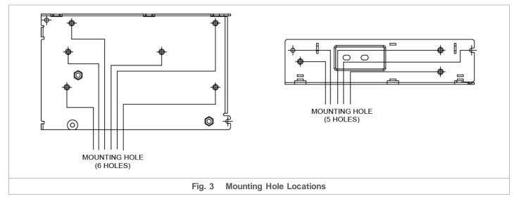
With reference to Fig. 3, the device should be mounted on a sturdy heat conducting surface with minimum of 4 mounting holes u sing M3 screw through the base or side mounting holes.
