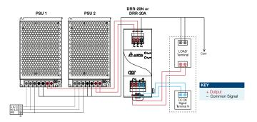
Fig. 5 Redundancy Operation Connection Diagram
