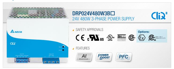
Delta Electronics extends the 3-phase models for its CliQ II DIN Rail Power Supply series with a 480W product offering 24V output voltage. The DRP024V480W3B□ is encased in a full aluminium body that can withstand shock (30G) and vibration (3G) according to IEC 60068-2 standard and operates over a wide temperature range from -25°C to +80°C.
